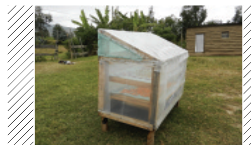
Fig. 94 Hand-made solar dryer
