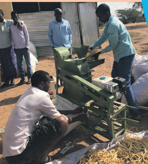
Prosopis for animal feed production – training in the use of hammer mills, Toghddeer region, Somaliland. Photo: Nicole Kenton.
